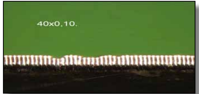
Anilox lines and chipping in low quality steel with few carbides.
